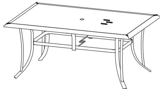
Once all of the bolts are in place, fully tighten the bolts. Turn the table right side up. Carefully place the glass (E) on the edge of the table (A). Ensure all connections are secure before use.
