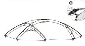
D) Snap J-hooks which are sewn on the screen house body over each roof pole to shape the screen house roof.
